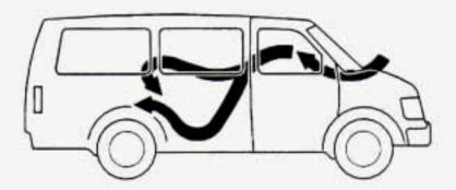
Your vehicle's ventilation system supplies outside air to the inside of your vehicle when it is moving. With the side windows closed, air will flow into the front air inlet grilles at the base of the windshield, through the vehicle and out the rear air exhaust valves. Outside air will also enter the vehicle when the heater or the air conditioning fan is running.
